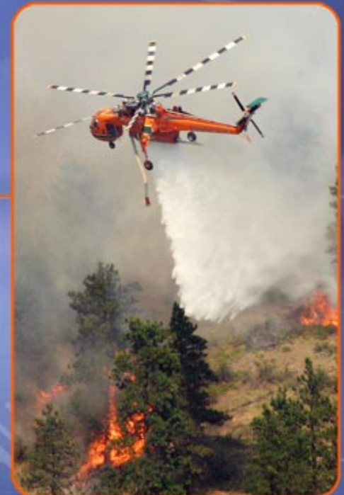
The 2,650 gallon (~10,000 liter) firefighting tank system features a metered flow multiple drop capability to fight fires within a variety of different fuel types. Refills accomplished in fresh water and salt water sources as fast as 30 seconds.
