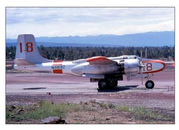
The Douglas A-26 saw it's first conversion in 1959 by Aero Atlas in Red Bluff Ca. By the mid 60s, somewhere between 50 and 60 A/B-26s were being used, some of them in California for a short time. The aircraft exhibited a 1,200 mile range coupled with a good airspeed and an initial 1,200 gallon capacity. By the late 60s and early 70s, a majority of the A-26s had either found their way to Canada, other non-tanker ownership or the scrap yards.
