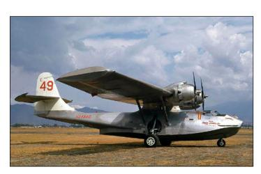
With experimentation in the 50s, the 1960s saw the widespread use of the Consolidated PBY both in the US and in Canada. Even thought is was a slow aircraft compared to several other tankers, it's low speed and 1,500 gallon capacity contributed to it's accuracy as a tanker. Being an amphibious aircraft, several of these had the capability of scooping water directly out of lakes to refill the tanks but more often than not, they remained land based.
