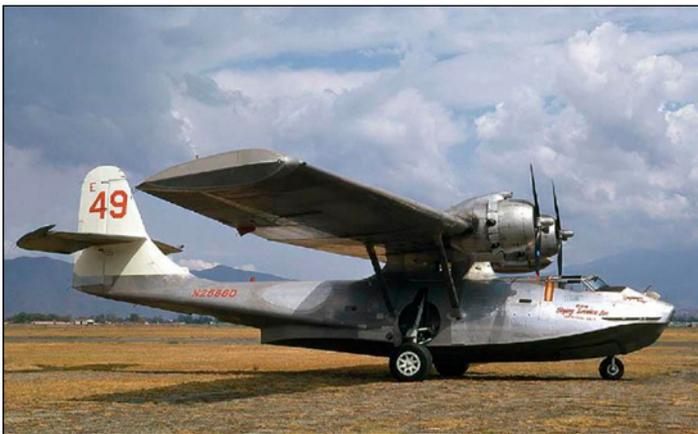
With experimentation in the 50s, the 1960s saw the widespread use of the Consolidated PBY both in the US and in Canada. Even though it was a slow aircraft compared to several other tankers, its low speed and 1,500 gallon capacity contributed to its accuracy as a tanker. Being an amphibious aircraft, several of these had the capability of scooping water directly out of lakes to refill the tanks but more often than not, they remained land based.
